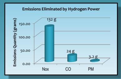
Shown in the graph above are the tailpipe emissions produced by generating 5kw of power with a diesel generator for an 8 hour day. Hydrogen Fuel cells completely eliminate these harmful emitted byproducts.
